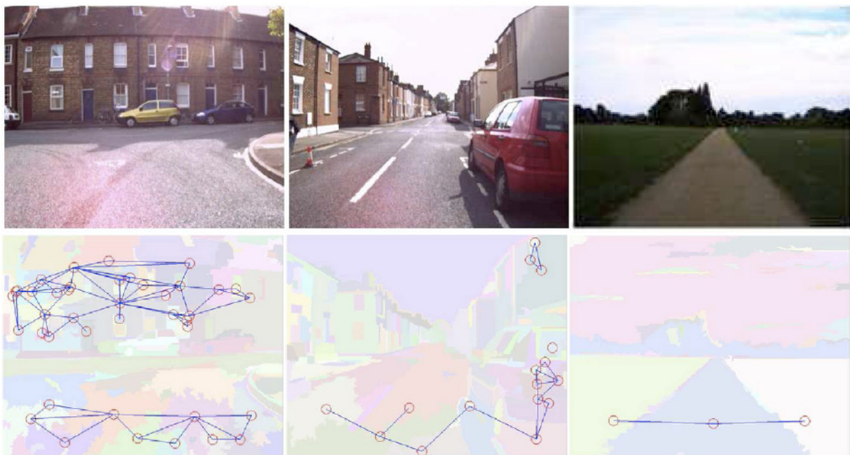
Figure 1: Typical graphs extracted from urban scenes as recorded by our mobile robot. Top: the original scenes. Bottom: the corresponding segmented images with the extracted graph overlaid. Circles indicate nodes, lines indicate edges. For images patches which are not marked as nodes no reliable geometry estimates could be extracted from the laser data. Reproduced from [1]
